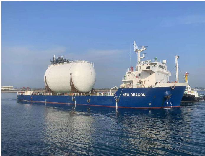
<Carrying LNG Tank (340MT) for bulk carrier's fuel tank >
